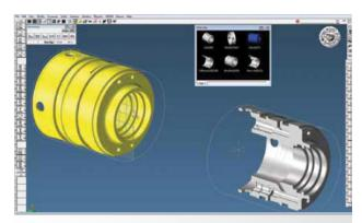
Before Kyle Vander Meyden programs a part with GibbsCAM, he uses its modeling capability to create a solid model to drive multi-axis MTM toolpath and for QA to program its CMMs. The drawing and solid modeling screen with active tool-processmachining palette and operations list enables seeing work on both main and subspindles.
