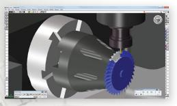
IMPROVED GOUGE AND TOOL INTERFERENCE DETECTION
